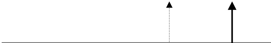
Figure 6. Interval Trigger that triggers when the interval falls within the selected range: T1=range's lower time limit; T2=range's upper limit. The broken upward pointing arrow indicates a potential trigger, while the bold one indicates where the actual trigger occurs — on the positive edge within the selected range.
